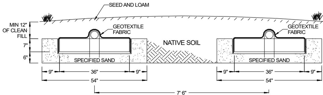
FIGURE 8: SECTION VIEW – TRENCH SYSTEM – SLOPING SITE
