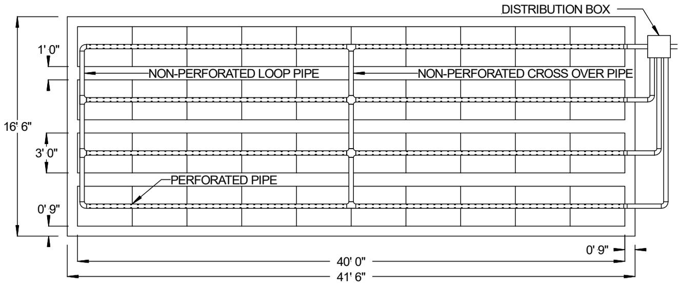
FIGURE 10: SECTION VIEW – BED SYSTEM EXAMPLE
